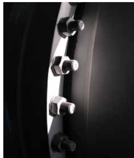
Wind turbine bolts with sensor
