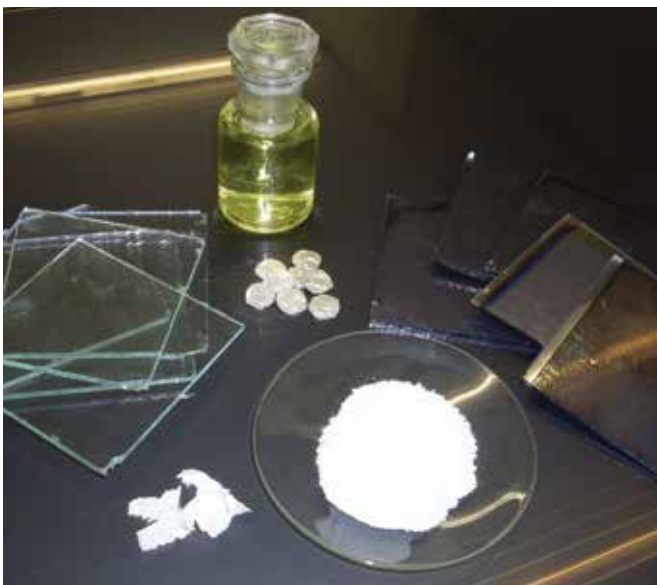
Raw material (black glass) and the possible products: clean glass, clean plastic foil flake (white, left), indium hydroxide (white powder), received from the yellow extraction solution, and last but not least, indium as metal
