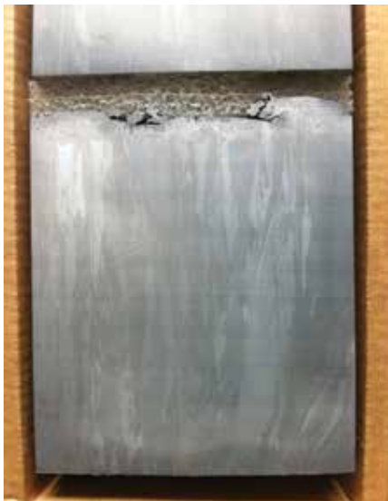
Pice (brick) as result of re-melting Si scrap after de-metallization
