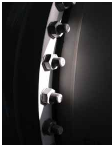
Wind turbine bolts with sensor
