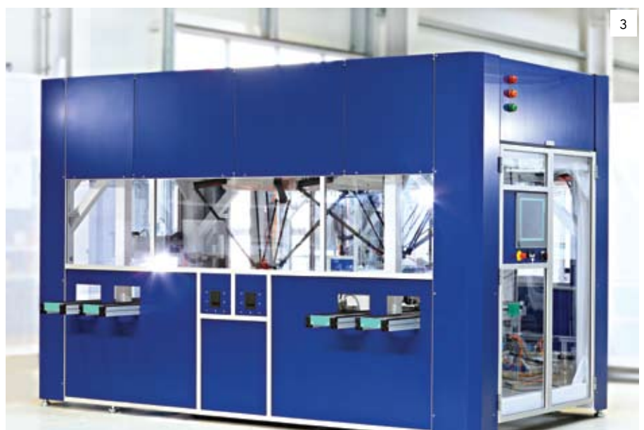
1. An AdeptSight image processing system controls several Adept Quattro S650 robots handling solar cells. 2. Using SCARA robots in the photovoltaic industry makes sense when speed and extremely accurate positioning of wafers and cells are required. 3. Two Adept Quattro s650 robotics systems in a cell handling solar wafers
